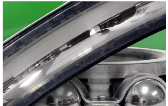
Figure 2: Taken from a failed motor, the "fluted" bearing race wall (top) resulted from VFD-induced bearing currents. Protected by an AEGIS™ SGR Bearing Protection Ring, the bearing race pictured above is undamaged.
